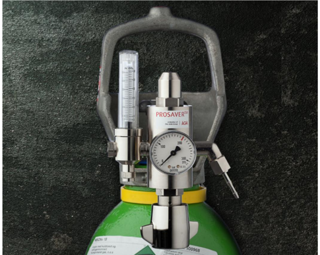
PROSAVER® is a regulator that reduces the cylinder gas pressure in two steps which results in a very smooth and stable flow of gas for MIG / MAG / TIG welding. It has an operating pressure of 2.5 bar and provides a gas flow between 2 - 30 L / min. PROSAVER® is recommended for advanced welding, where the demands for quality, accuracy and economy must be ensured.
